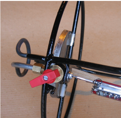
Install the fuel valve and heater pipe
